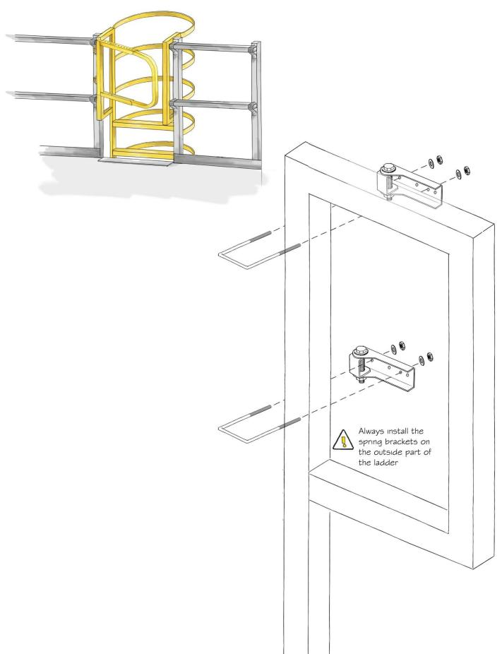
(The top of the gate must be between 41"- 42" high from the top of the deck)
